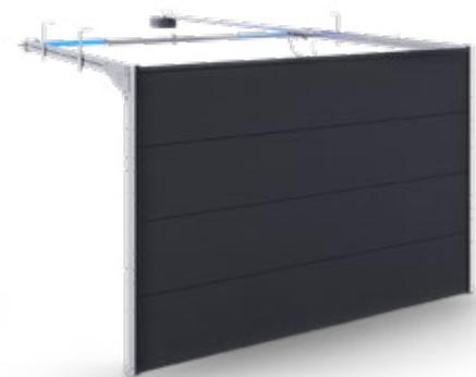
Location of the torsion springs at the rear part of the door allows it to be mounted to the garage opening with a lower lintel. In this case, it is sufficient for the lintel to be 85 mm (115 mm for an electric drive). Maximum lifting capacity up to approx. 195 kg.
