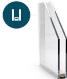
A single-chamber glazing unit consisting of two glass panes. It is a standard for basic window and door systems. In the space between the panes, created by the spacer bar, there is mainly argon (90%), which additionally reduces the  $U_g$  heat transfer coefficient.
