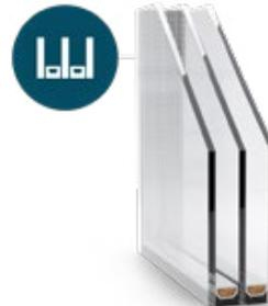
A triple glazing unit consisting of three glass panes. It is a standard for window and door systems with increased thermal properties. In the space between the panes, created by the spacer bar, there is mainly argon (90%), which additionally reduces the  $U_g$  heat transfer coefficient.
