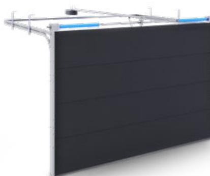
Torsion springs are dedicated to large-size garages doors. They lift much more weight than the tension springs. Installation of doors with torsion springs at the front is possible when the lintel height is at least 200 mm. The maximum weight of the gate is about 195 kg.
