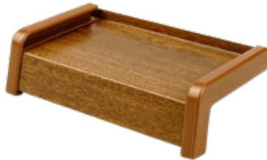
A galvanized steel windowsill covered with PVC foil. Made of 0.7 mm thick sheet metal with 275 g / m<sup>2</sup> zinc coating. It is possible to make a windowsill with a maximum length of 6 m, and the range of their width is: 100-400 mm.
