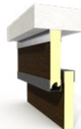
An artificial lintel that masks the structure, using door panel materials.
