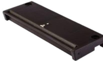
A rebate vent, which is placed in the inner part of the frame, makes it almost invisible when the window is closed. This allows air to circulate at the point of installation. Air flow (for two diffusers) at 10 Pa:  $5 \text{ m}^3 / \text{h}$ . Acoustic attenuation:  $D_n, e, w = 34 \text{ dB}$
