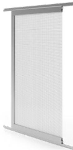
Ideally suited for zero-threshold sliding door systems, as it is installed on tracks at floor height, without a threshold. Rigid construction thanks to folded inner corners. The recessed inner side replaces the handle. Width 20 mm.
