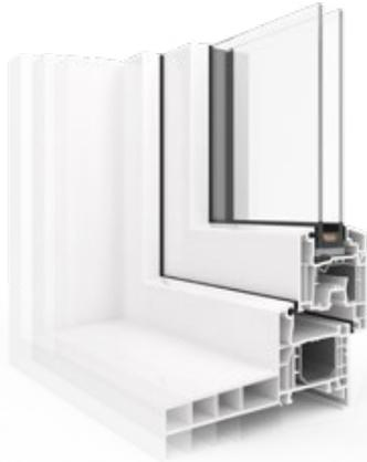
Frame profile designed for wall mounting with a thermal insulation layer. The availability of different widths of the masking element forming the windowsill allows for the use of profiles with different installation depths.
