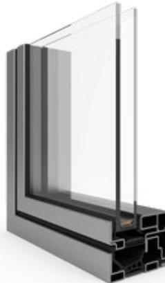
The profile is made of steel on the inside and outside. In the central part, there is a thermal break, which significantly increases the thermal insulation of the profile.
