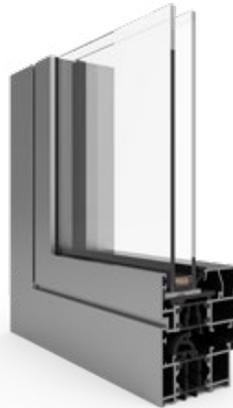
The profile is made of aluminum on the inside and outside. In the central part, there is a thermal break, which significantly increases the thermal insulation of the profiles.
