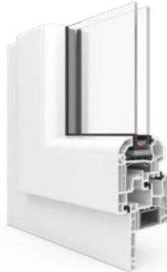
A profile that enables the installation of windows in existing buildings, without the need to disassemble the old frames. The fin covers the old frame inside the building, and special additional profiles mask it from the outside.
